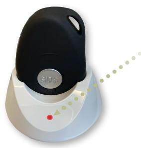
Once you receive your Sidekick, plug its charging cradle into an outlet. Place the Sidekick in the cradle with the SOS help button facing forward. Ensure your Sidekick is firmly pushed into the charging cradle to initiate charging. When charging properly, the RED light on the cradle will turn on and the Sidekick will announce "Charging."
